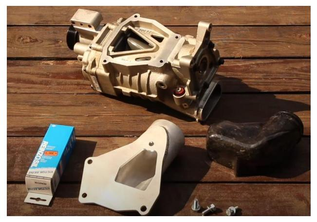
Step one is to service the Super Charger oil in front and rear oil fill holes using the right oil 40 ml oil for front and 145 ml oil for rear
