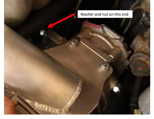
Now you can tighten the rear bolt abd the bottom two bolts on the front bracket but not the long bolt for the tensioner
