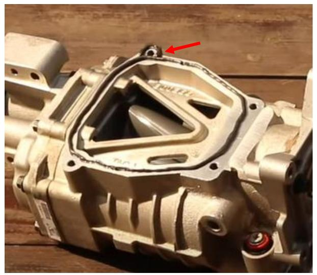
The one bolt in the outlet pipe will require you to apply some lock tight to the threads before you insert it. To insure you do not drop ANYTHING into the super charger insert a CLEAN rag in to the pipe first this will save you the pain of ruining your super charger.
