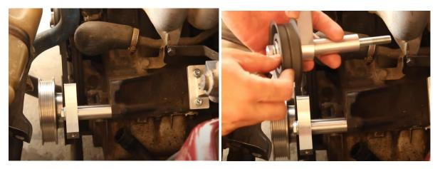
Preasembly of 3<sup>rd</sup> arm spacer with pulley and spacer
