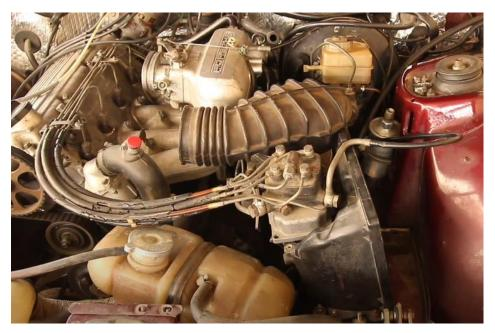
Now you will need to rotate the engine to top dead center using the markes on the pulley and oil pump housing as in the picture.
