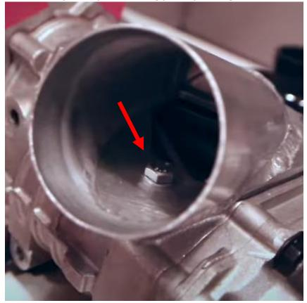
Tighten the bolt with the locktite and remove the rag. Now tape over the opening for saftety.
