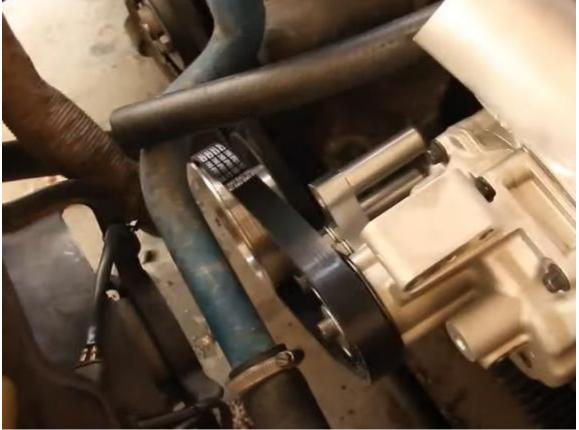
next step is to place the tensioner on top of the belt and then insert the bolt thru the tenisioner and spacer then insert the bolt for the top mount arm (you will tighten this bolt very last)
