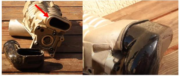
Set Super charger aside for 4 hours in order for the sealant to cure
