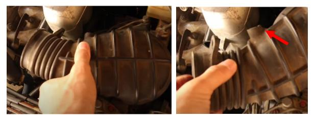
Now rotate the rubber intake to connect to the new inlet and using a little oil on the rubber to lube up both ends so that installing will be easier carefully slide on to the new outlet pipe. You may want to loosen the long M6 bolt a bit but be very carefull as the new 3D printed pipe is brittle, then tighten the M6 bolt just snug so you don't crack the new outlet pipe.
