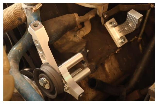
Only the rear bracket bolts should be tight at this point. You will need the front bolt loose to finish the install. On the body there is a bracket with a rubber insulation block that you need to loosen and turn 90 degrees see picture below.
