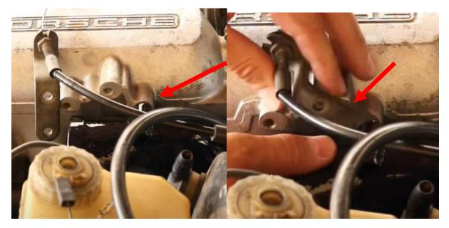
The throttle bracket will sit between the manifold and the outlet pipe and be secured in place using the long M6 bolt from kit.
